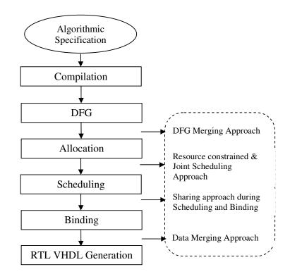
Figure 1. HLS Design Flow with Proposed architecture design
