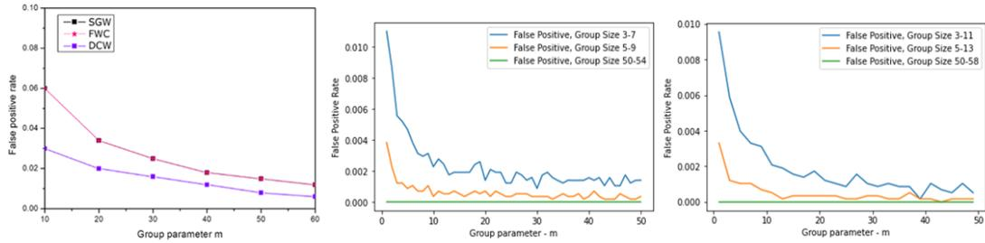
Figure 8 (Right and Middle image) it can also be seen that the false rate decreases as the group parameter increases. In [15], the lower bound 'L' is 50, whereas in this experiment the value for 'L' is very low for which the false rate tends to zero.
