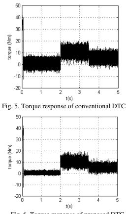
Fig. 6. Torque response of proposed DTC
