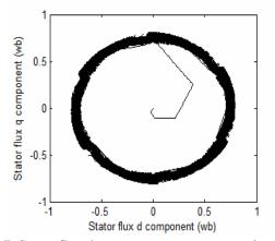
Fig. 7. Stator flux d-q components on conventional DTC
