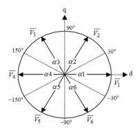
Figure 1. Inverter voltage vectors and sectors
