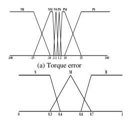
(b) Initial value of stator flux reference
