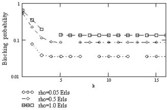
Figure 4: Blocking Probability as a function of the fold number under different offered traffic (N=50, n=14, q=5,  $\theta = .31$ )
