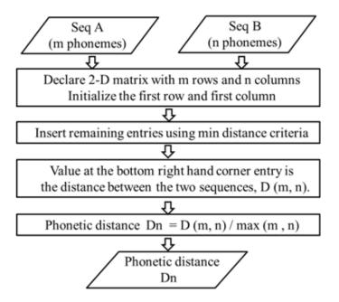
Figure 3: Flow chart for DPW algorithm
